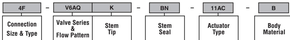
**Oxygen Cleaning** – Add the suffix **-C3** to the end of the part number to receive valves cleaned in accordance with ASTM G93 level C, class 500. This ASTM details cleaning methods and cleanliness levels for materials and equipment used in oxygen-enriched environments. **Example:** 4A-V4AQ-EPR-SSP-C3
