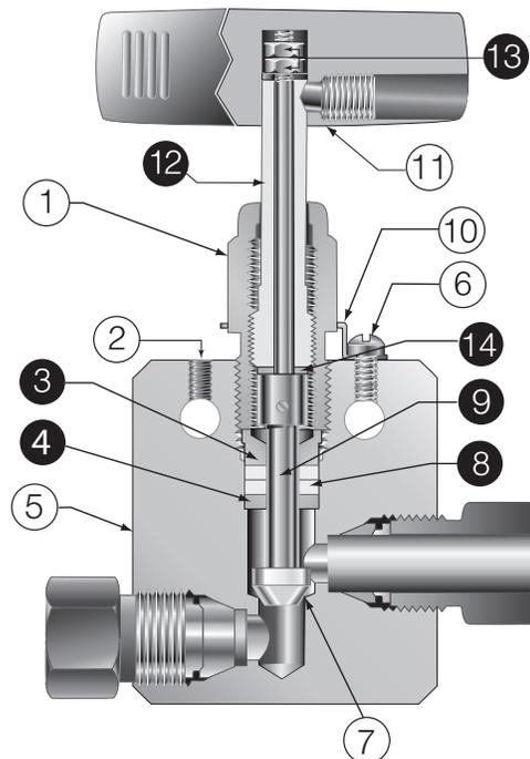
Inlet is typically under the seat (from left side in drawing above) however valve can be used bi-directionally. Inlet is shown to keep pressure trapped under seat in closed position (preferred).
