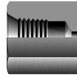
**M** – ANSI/ASME B1.20.1 external pipe threads
