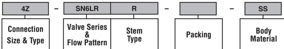
**Note: Handles:** SN6 valves with R-Stem are standard with 316 SS T-bar handles. SN6 valves with K-Stem are standard with round anodized aluminum handles, 1.00 inch diameter. SN6 valves are not panel mountable.
