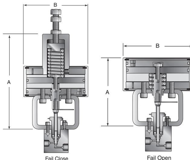
NOTE: Air inlet for Fail Close operation is located in the back, opposite the front of valve. For other locations, consult factory. Holes supplied in yoke bracket for mounting.
